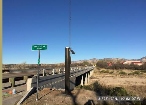
This ALERT precipitation and radar stage station was installed for Santa Cruz County on January 12, 2016 on the Santa Cruz River at State Highway 82 near Nogales, Arizona.
