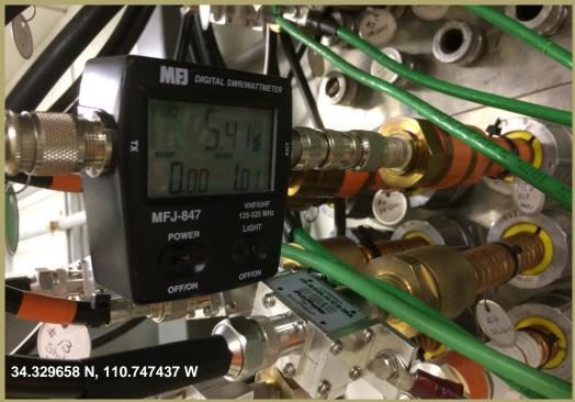
Hint: see the output, reflection and SWR calculation in the display.
