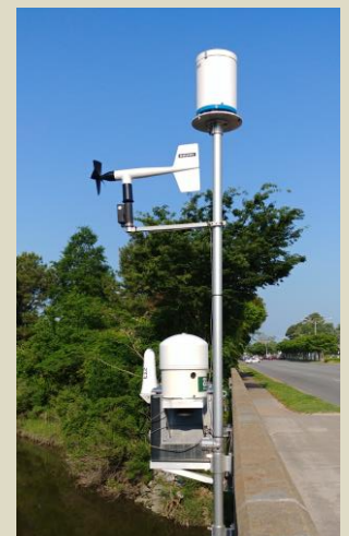
Figure 1- A typical U.S. Geological Survey stage (water level) station with accompanying meteorological sensors.
