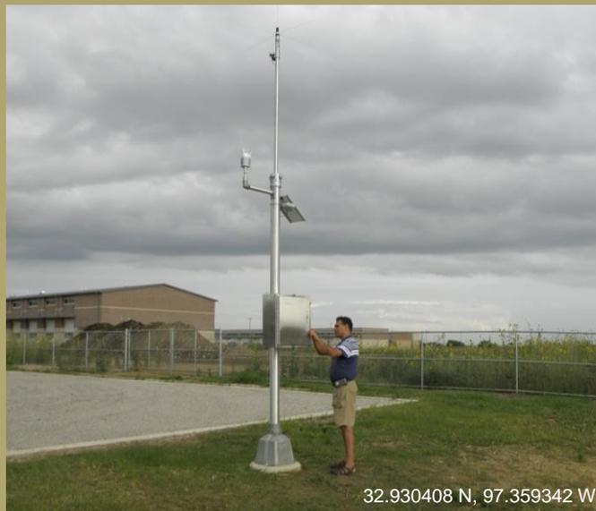
Ranjan Muttiah (City of Fort Worth, Stormwater Management) secures the enclosure of the city's first ALERT2 gauging station. This multi-parameter station, located at the City's Northside Service Center, is equipped with a Vaisala WXT536 multi-parameter weather sensor (precipitation, temperature, humidity, pressure and wind speed/direction). One third of new planned stations will include tipping bucket precipitation sensors for data quality comparison purposes.
